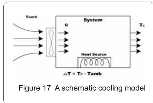
Figure 17 A schematic cooling model
