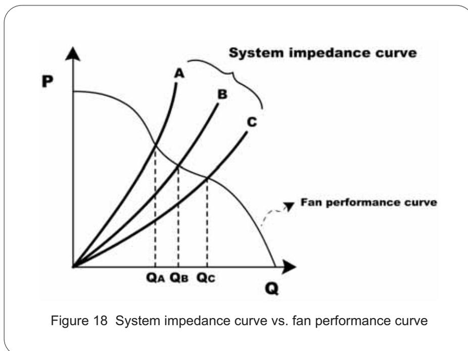
Figure 18 System impedance curve vs. fan performance curve
