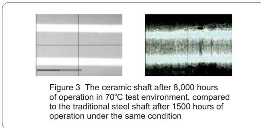
Figure 3 The ceramic shaft after 8,000 hours of operation in 70°C test environment, compared to the traditional steel shaft after 1500 hours of operation under the same condition
