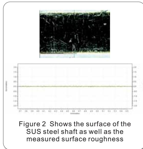
Figure 2 Shows the surface of the SUS steel shaft as well as the measured surface roughness
