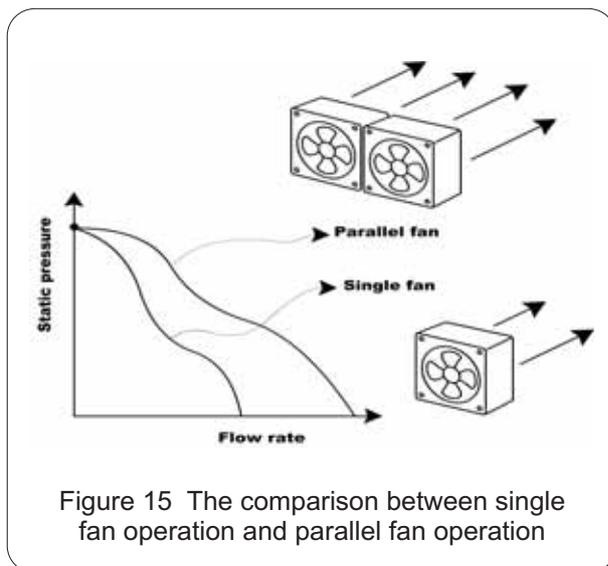
Figure 15 The comparison between single fan operation and parallel fan operation
