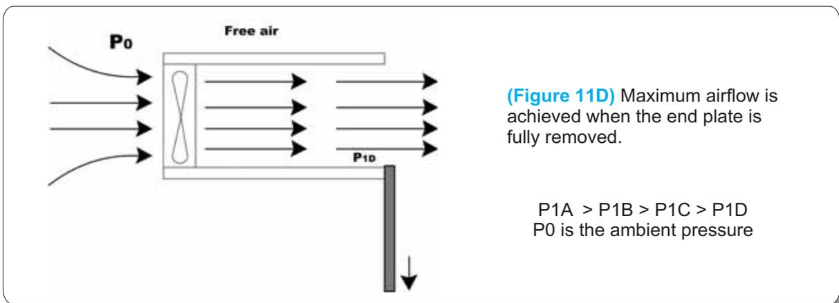
As the end plate is fully removed, the tube pressure becomes minimum, and no resistance within the tube. (assuming Non-viscous flow, no friction and no boundary layer closed to the wall).
