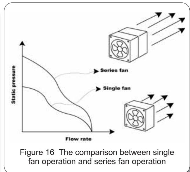
Figure 16 The comparison between single fan operation and series fan operation
